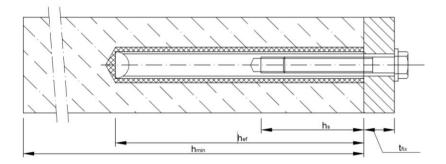
$t_{\text{fix}}$  = thickness of fixture
