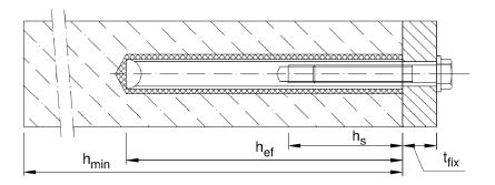
$t_{fix}$  = thickness of fixture
